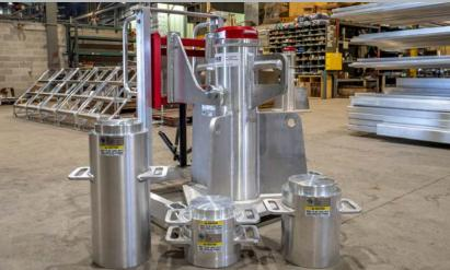
The EHDS stand system is a very versatile equipment stand system that offers a base stand and adjustment caps that range in height from 2" - 22". The stands are available in two capacities, 65 ton and 125 ton per stand. The base height is available in two sizes 17.75" and 37.75". The stands come c/w fork pockets and dolly lifting knobs. Most systems utilize a lifting dolly on wheels. Achieve all your height requirements in one simple system.
