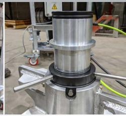
The BDHJ-35 offers a safe solution to lifting larger pieces of Mining, Construction or Forestry Equipment. Capacity of 70 ton (2-35 ton Jacks) or 140 ton (4-35 ton Jacks). Ideal for lifting large wheel loaders, dozers, excavators, scoop trams, haul trucks and forestry equipment.
