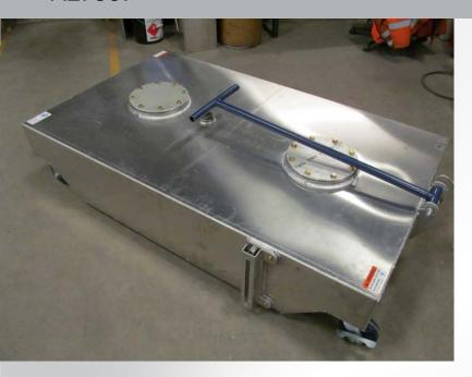
Constructed as a sealed and vented tank to reuse the antifreeze, our 140 gal (529 L) low profile cart comes with 2" (51 mm) intake and discharge ports, 2 clean-out ports and sight glass. A heavy duty handle, four oil resistant swivel casters make it easy to maneuver. Fits under equipment of any size.
