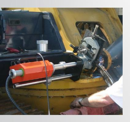
The BOA portable welder system saves both cut, welding time, and machining time with smooth, high-quality welders on internal and external diameters.
