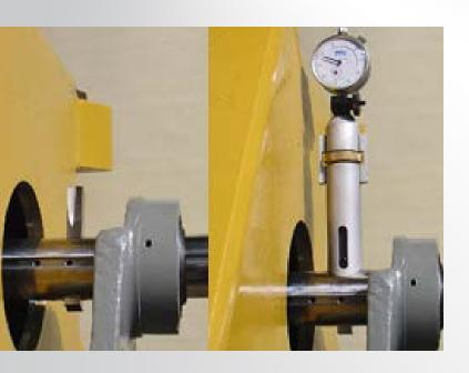
2" machine packages. The unique B & D DTA provides accurate adjustment to the cutting depth of the HSS or carbide tool bit to within a hundredth of an inch. Using the DTA is easy. Just slip it over the tool bit and rest it against the boring bar. Clamp the tool bit to the DTA by tightening the set screw.
